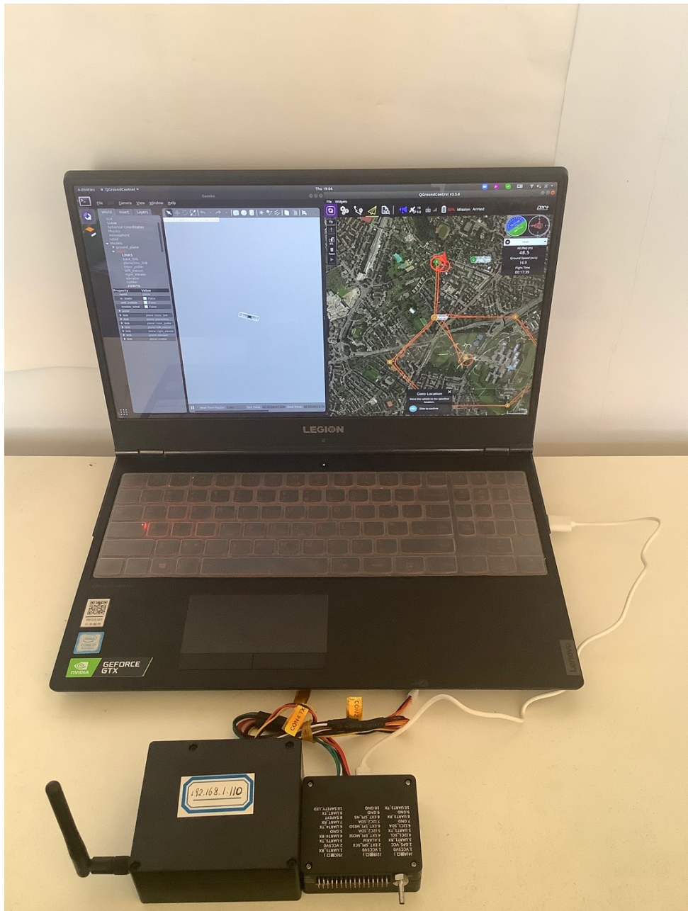
Figure 2.16: Setup for hardware-in-the-loop experiments: a PX4/Raspberry Pi 3B+ controller uses a MAVROS node to share data with a Gazebo 3D simulator
