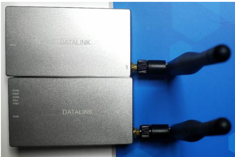
Figure 6.4: The Microhard pDDL900 datalink
