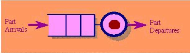
This is a single stage manufacturing process modeled as a HYBRID SYSTEM:
