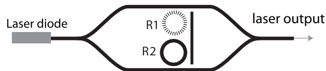
Figure 5: Schematical representation of the designed laser, with a wavelength tunabilty of 44.6 nm. R1=50 \mu\text{m} , R2=55 \mu\text{m} .
