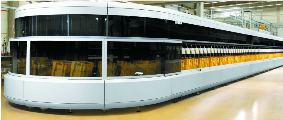
Figure 1.1: Sorting part of a flat sorting machine. Picture source: Siemens AG, Infrastructure Logistics, 2009.
