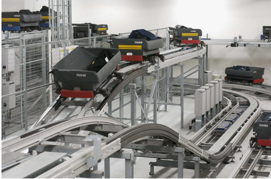
Figure 1.3: DCVs running on a network of tracks. Photo courtesy of Vanderlande Industries.
