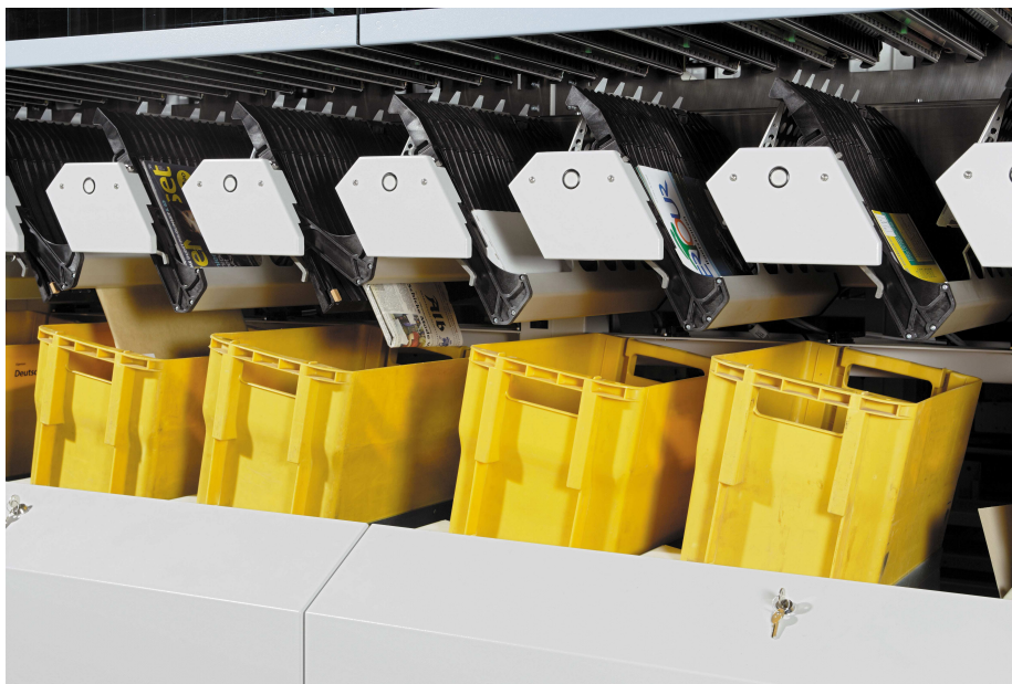
Figure 1.2: Dropping a flat into a bin. Picture source: Siemens AG, Infrastructure Logistics, 2009.
