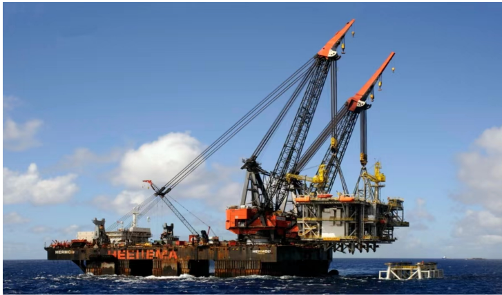
Figure 1.2: Heavy-lift vessel with multiple cranes (source: Heerema Marine Contractors)
