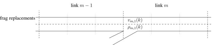
Figure 3.3: When there is an on-ramp connected to the freeway the speed  $v_{m,1}(k)$  in the first segment of link m is reduced by merging phenomena according to (3.7).
