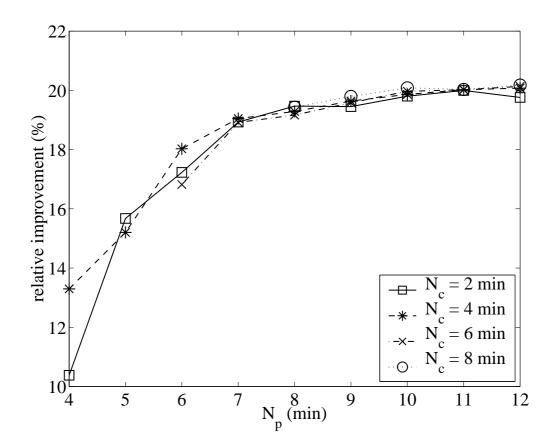
Figure 6.17: The relative improvement of the performance (TTS) for scenario 1 in the real-valued, unconstrained case compared to the 'no control' case as a function of  $N_{\rm p}$  for several values of  $N_{\rm c}$ . The sensitivity to  $N_{\rm p}$  is much higher than that to  $N_{\rm c}$ .
