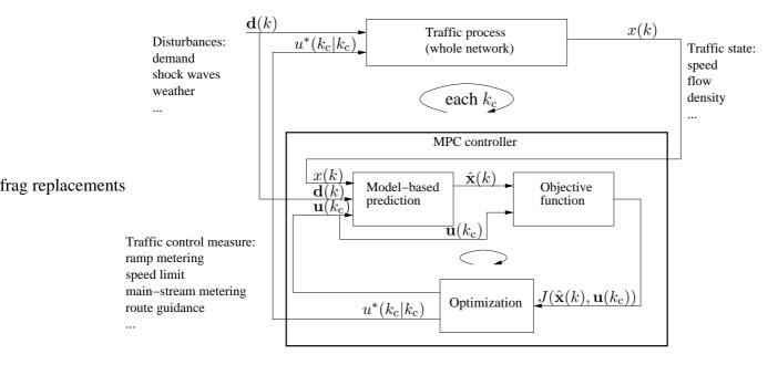
Figure 4.4: The MPC scheme for traffic control.
