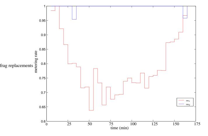
*Figure 7.6: Metering rates of the metering systems at ramp link*  $L_6$  ( $rm_1$ ) and ramp link  $L_{12}$  ( $rm_2$ ).
