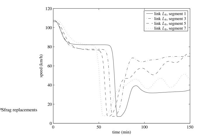
Figure 7.3: Evolution of the mean speed on some segments of link  $L_8$  in the 'no control' case. When no control measures are activated, the shock wave propagates through link  $L_8$ , and speed on this decreases significantly.
