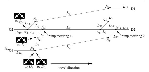
Figure 7.2: The traffic network of the case study consists of two origins  $O_1$ ,  $O_2$ , and two destinations  $D_1$ ,  $D_2$ . The network contains a freeway (consisting of links  $L_{17}$ ,  $L_4$ ,  $L_8$ ,  $L_9$ , and  $L_{14}$ ), and secondary roads (consisting of the other links). There are four DRIPs and two on-ramp metering installations (indicated by the symbol RM).
