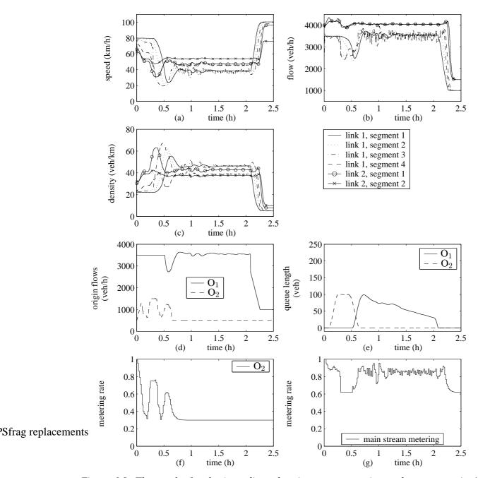
Figure 6.9: The results for the 'coordinated main-stream metering and ramp metering'. The behavior of the main stream metering is similar to behavior of the speed limits in the 'coordinated speed limits and ramp metering' case.
