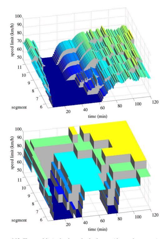
Figure 6.15: The speed limits for the real-valued case without safety constraints and  $N_{\rm p} = 10$ ,  $N_{\rm c} = 8$  (top). The speed limits for the discrete ('ceil') case with safety constraints and  $N_{\rm p} = 10$ ,  $N_{\rm c} = 8$ .
