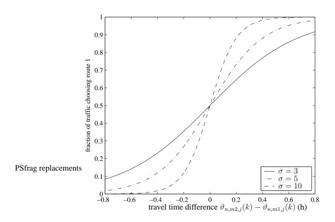
Figure 7.1: An example of the resulting splitting rates as a function of the travel time differences according to the logit model. It is assumed that  $\vartheta_{n,m2,j}(k) = I h$ .
