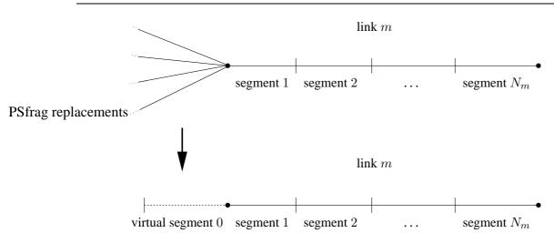
Figure 3.6: A node with one leaving link m and several entering links. The speeds in the last segments of the entering links are aggregated in the virtual upstream speed  $v_{m,0}(k)$  according to (3.10).
