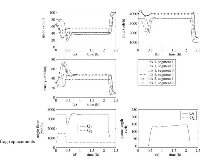
Figure 6.5: The simulation for the 'no control' case. The high demand on the on-ramp causes a congestion that remains existing until the main-stream demand drops to a low value.
