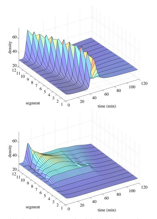
Figure 6.14: The shock wave propagates through the link in the 'no control' case (top). In the 'coordinated control' case, the shock wave disappears after approximately 90 min (bottom).
