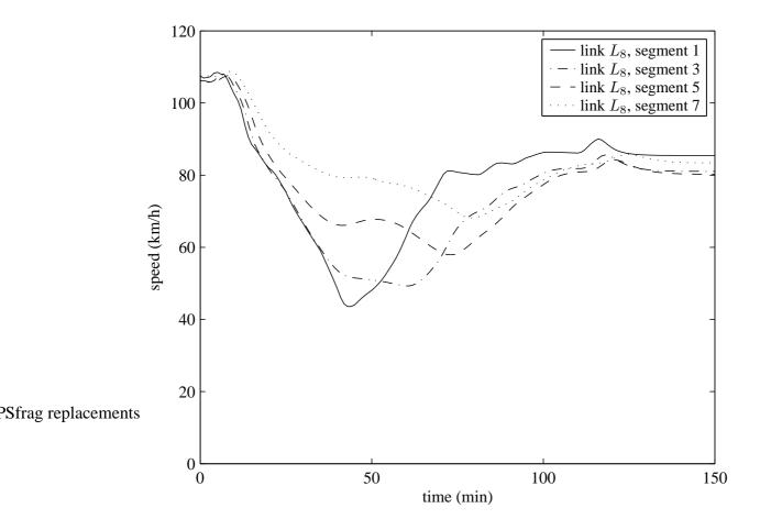
Figure 7.4: Evolution of the mean speed on the segments of link  $L_8$  when route guidance and ramp metering is applied. Ramp metering and rerouting results in more traffic choosing alternative routes via the secondary roads, which leads to less traffic on link  $L_8$  and increased speeds with respect to the 'no control' case.
