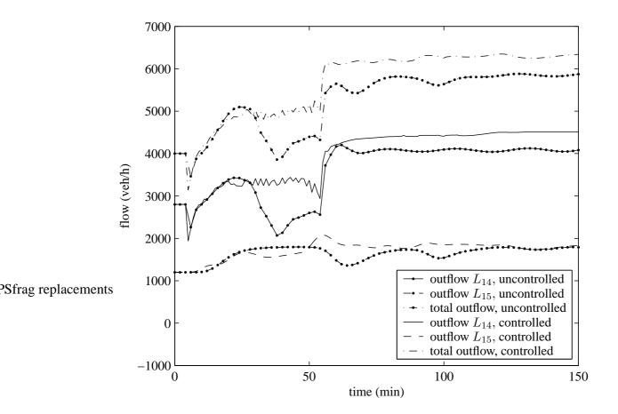
Figure 7.5: Evolution of the outflow of the exit links  $L_{14}$  and  $L_{15}$  and the total outflow in the uncontrolled and controlled cases. The outflow of the controlled case is higher.
