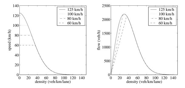
Figure 3.9: The speed-density and flow-density relationships of the new speed limit model proposed in this thesis, (with  $v_{\text{free},m} = 125 \text{ km/h}$ ,  $a_m = 1.867$ ,  $\rho_{\text{crit},m} = 30 \text{ veh/km/lane}$ , and  $\alpha = 0.$ )
