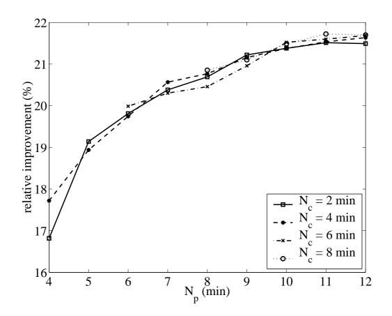
Figure 6.21: The relative improvement of the performance (TTS) for scenario 2 in the real-valued, unconstrained case compared to the 'no control' case as a function of  $N_{\rm p}$  for several values of  $N_{\rm c}$ . The sensitivity to  $N_{\rm p}$  is much higher than that to  $N_{\rm c}$ .
