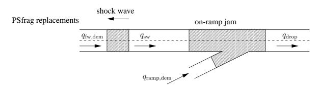
Figure 5.7: The shock wave upstream from the on-ramp jam feeds the on-ramp with a constant demand of approximately  $0.7q_{cap}$ .
