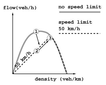
Figure 6.1: When traffic on the main road is in state 1, then it is nearly unstable and even a small flow from the on-ramp can cause a breakdown. Speed limits change the state from 1 to somewhere between 2 and 3, and change the shape of the fundamental diagram from the solid gray line to the dashed black line. The decrease of flow creates some space for the on-ramp traffic.
