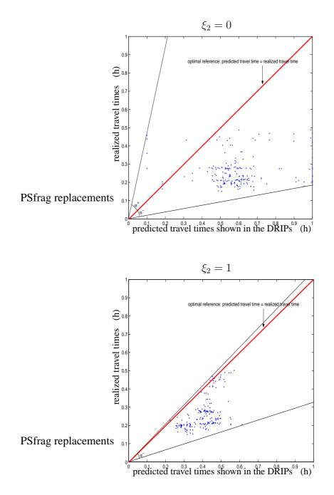
Figure 7.7: Plot of the travel time prediction error in case the weighting factor  $\xi_2$  for the prediction error term in the objective function is set to 0 (top) and to 1 (bottom). The angles  $\alpha^+$  and  $\alpha^-$  are representative for the maximum relative errors of the shown travel times.
