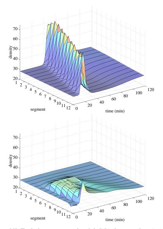
*Figure 6.19: The shock wave propagates through the link in the no control case (top). In the coordinated control case, the shock wave disappears after approximately 2 h (bottom).*
