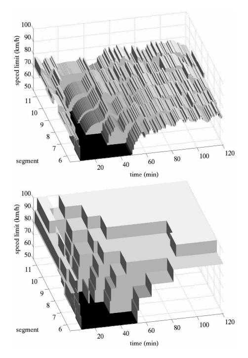
Figure 6.20: The speed limits for the real-valued case without safety constraints and  $N_{\rm p} = 11$ ,  $N_{\rm c} = 8$  (top). The speed limits for the discrete (ceil) case with safety constraints and  $N_{\rm p} = 11$ ,  $N_{\rm c} = 8$ . For the purpose of visibility, the travel direction is opposite to that in Figure 6.19.
