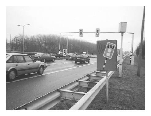
*Figure 2.1: Ramp metering at the A13 at Delft in The Netherlands. One car may pass per green phase. To prevent red-light running the control is enforced.*
