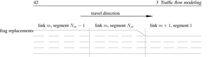
Figure 3.4: When there is a lane drop the speed  $v_{m,N_m}(k)$  in the last segment of link m is reduced by merging phenomena according to (3.8).
