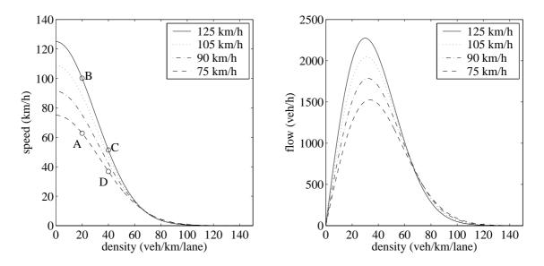
*Figure 3.7: The speed-density and flow-density relationships for model 1. The speed limit of 125 km/h corresponds to the unlimited case.*
